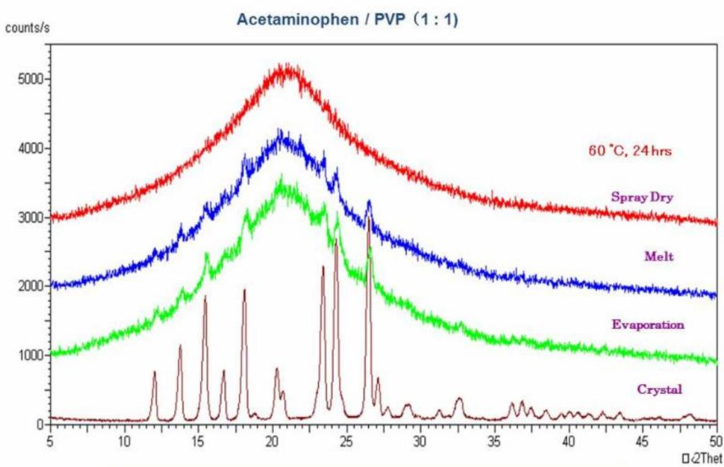
The XRD data above shows comparison study results of various solid dispersion methods using PVP as the polymer to spray dry acetaminophen, subsequently stored for 24 hours at 60°C before the analysis. The solid dispersion prepared by spray dry method indicated halo pattern in contrast with solid dispersions prepared by melt method and evaporation method, which indicated slight crystalline peaks. The study demonstrates that spray drying is more stable than other methods.
